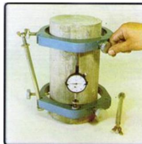
SC-500 MODULUS OF ELASTICITY IN CONCRETE TEST SET For measuring average axial deformation of concrete cylinder sample during compression test, cast aluminium, dial indicator 0.001 x 5 mm. Dimension (l x w x h) = 30 x 30 x 35 cm.
