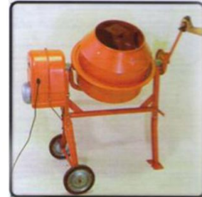
SC-610 LABORATORY CONCRETE MIXER For mixing trial batches of concrete for mix design, Approx 70 ltr capacity, 4 mixing blades, welded steel frame, 2 wheels for easy movement, electromotor 1/3 HP, 220 V-AC, 1 Phase. Dimension (l x w x h) = 20 x 20 x 30 cm.
