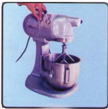
MORTAR MEXER Bench model ,electric 220 V-AC, supplied complete with beaters. Type Part Name Specification Mortar Milixer 5 litre capacity Mortar Mixer 10 litre capacity
