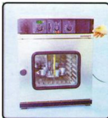
SI -220 LOSS ON HEATING / THIN-FILM TEST For determining the loss in mass (exclusive of water) of asphaltic compound after heating.
