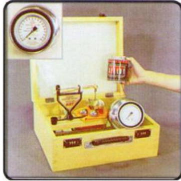
SS -430 SPEEDY MOISTURE TESTER For determining the moisture content of soil by means of calcium carbide gas pressure meter.
