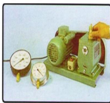
Manometer, Vacuum Manometer, Vacuum Pump
