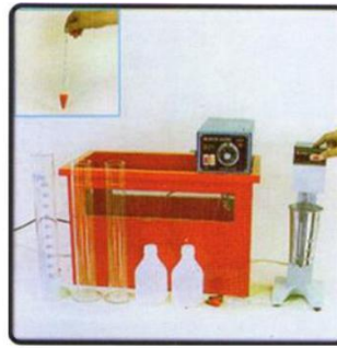
SS -330 A HYDROMETER ANALYSIS TEST SET For determining grain size distribution of fine soil sample ASTM D-422 / AASHTO T-88
