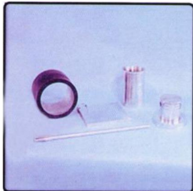
SA -760 AGGREGATE CRUSHING VALUE APPARATUS For determining the crushing properties of bulk aggregate applying 400 kN load over a period of 10 minutes.
