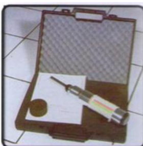
SC-550 CONCRETE TEST HAMMER ASTM C-805 For rapid quality control of concrete work, with built in pointer scale and graph for various angle. Dimension (l x w x h) : 15 x 15 x 40 cm.
