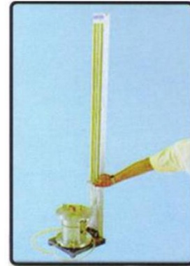
SS -390 A COMPACTION PERMEAMETER TEST SET For determining coefficient of permeability of soil sample
