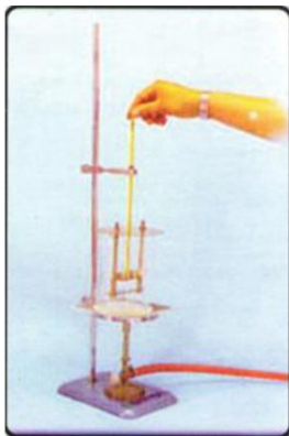
SI -210 SOFTENING POINT TEST SET For determining softening point of asphalt and tar using the ring and ball method
