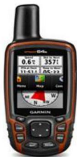
Geodetic global positioning system (G-GPS) Garmin GPSMAP 64S Physical dimensions : 2.4" x 6.3" x 1.4" (6.1 x 16.0 x 3.6 cm) Display size, WxH : 1.43" x 2.15" (3.6 x 5.5 cm); 2.6" diag (6.6 cm) Display resolution, WxH : 160 x 240 pixels Display type : transfective, 65-K color TFT, transfective Weight : 8.1 oz (230 g) with batteries Battery : 2 AA batteries (not included); NIMH or Lithium recommended Battery life : 16 hours Water rating : IPX7 High-sensitivity receiver : YES Interface : high-speed USB and NMEA 0183 compatible Barometric altimeter : YES Electronic compass : Yes (tilt-compensated 3-axis) Unit-to-unit transfer (shares data wirelessly with similar units) : YES MAPS & MEMORY Basemap : YES Ability to add maps : YES Built-in memory : 4GB Accepts data cards : microSD™ card (not included) Custom POIs (ability to add additional points of interest) : YES Waypoints/favorites/locations : 5000 Routes : 200 Track log : 10,000 points, 200 saved tracks OUTDOOR FEATURES Automatic routing (turn by turn routing on roads) : YES Geocaching-friendly : Yes (Paperless) Custom maps compatible : YES Hunt/fish calendar : YES Sun and moon information : YES Tide tables : Yes (with optional Bluechart) Area calculation : YES Picture viewer : YES Garmin Connect™ compatible (online community where you analyze, categorize and share data) : YES
